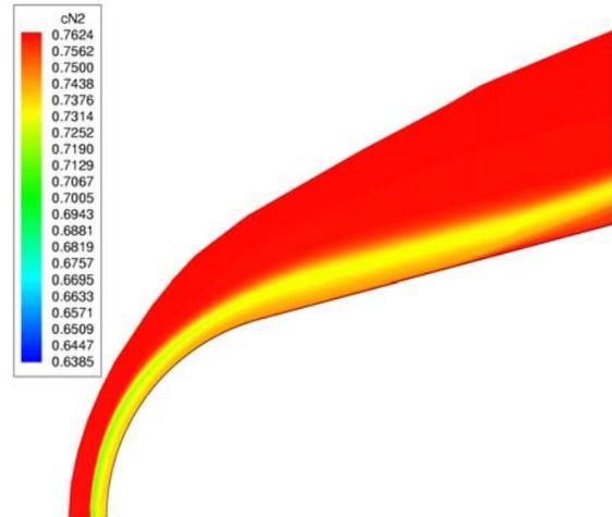
Figure 44 N<sub>2</sub> concentration at  $M_\infty=12.9$  for catalytic wall assumption.
