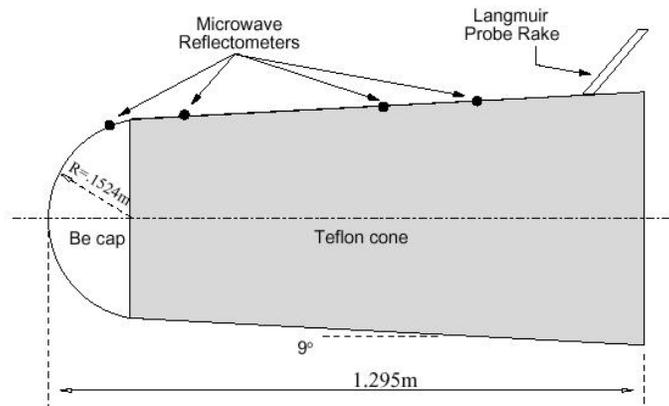
**Figure 9 Langmuir probe/RAM C flight test.**
