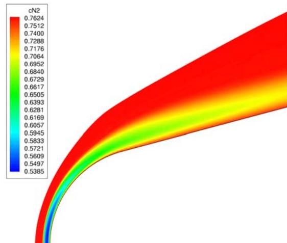
Figure 45 N<sub>2</sub> concentration at  $M_\infty=22.5$  for catalytic wall assumption.
