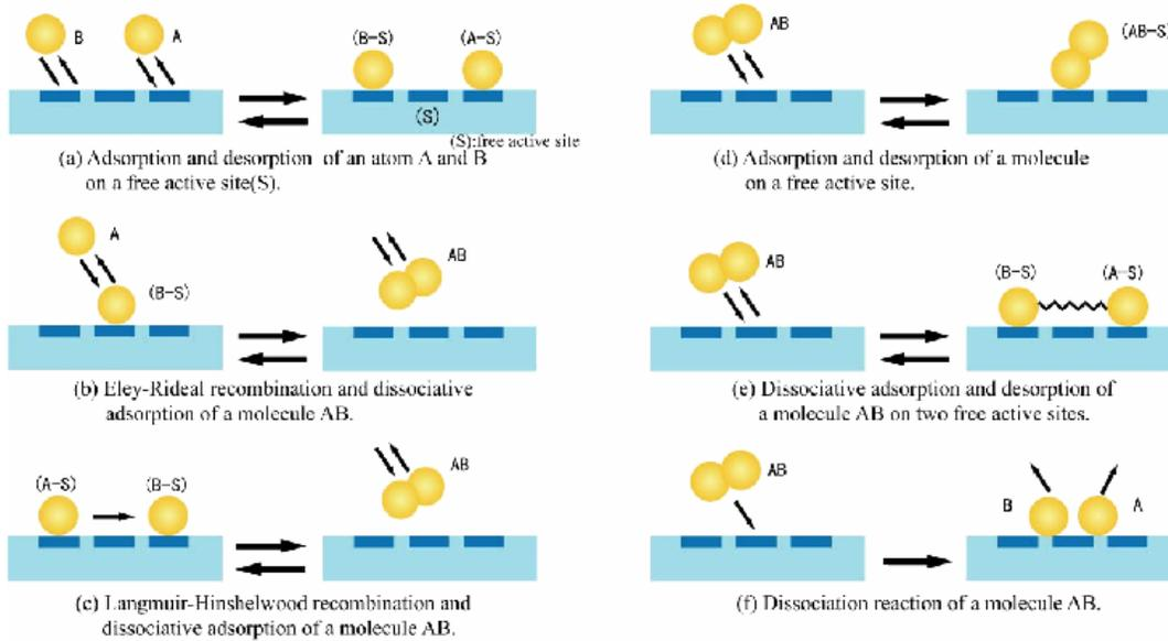
Figure 12 Chemical Processes in Heterogenous Catalysis on Surface
