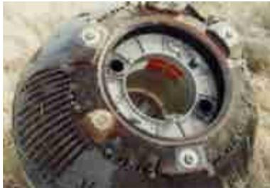
Spherical capsule to test innovative Surface Protected Ablator thermal protection
