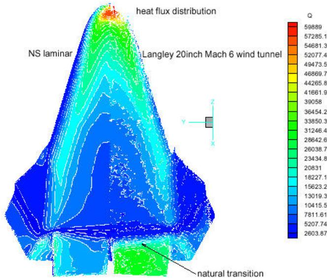
**Figure 6 X-38 heat flux distribution at Mach 6.**
