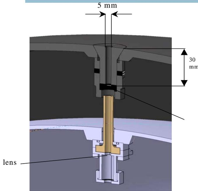
sapphire window: thickness 3 mm, diameter 14 mm
