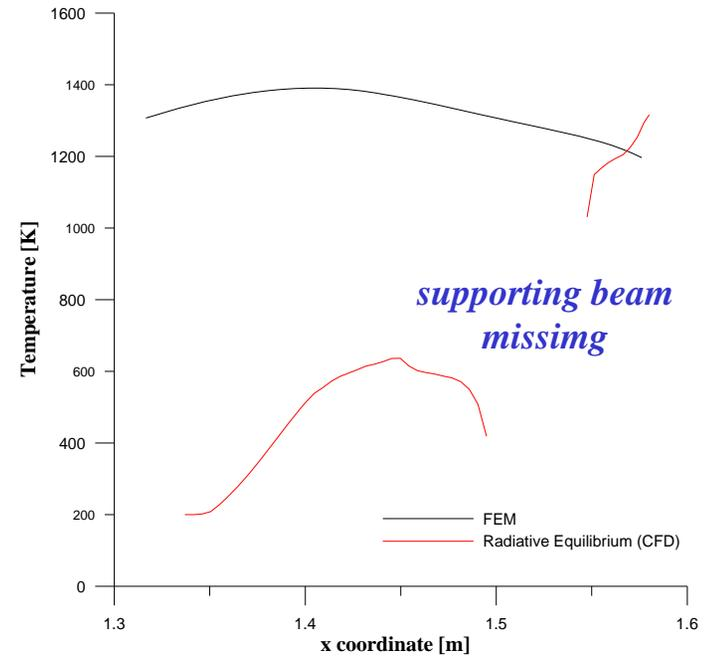
Because of *conduction and radiation* the backside temperature is much higher than the corresponding radiative equilibrium wall temperature.
