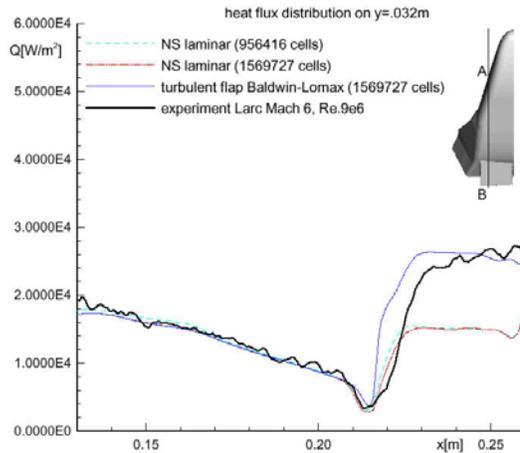
**Figure 7 X-38 flap heating at Mach 6.**
