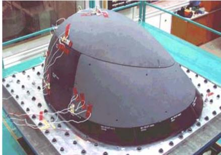
TETRA nose assembly and thermo-mechanical nose tests
