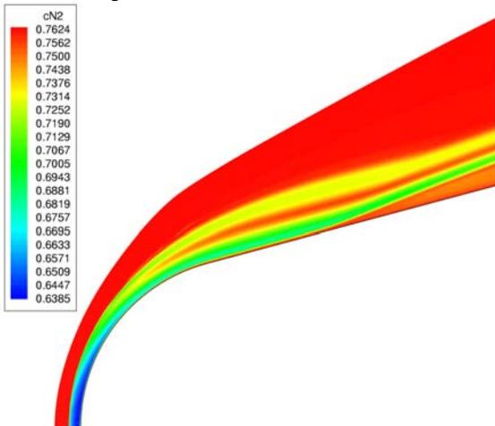
Figure 43 N<sub>2</sub> concentration at  $M_\infty=17.0$  for catalytic wall assumption.
