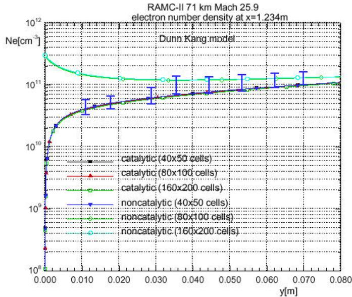
Figure 11 RAM C flight rebuilding with Dunn-Kang model.
