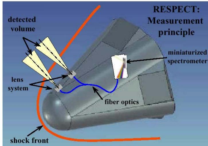
**Figure 48 RESPECT mounted on EXPERT (courtesy IRS).**
