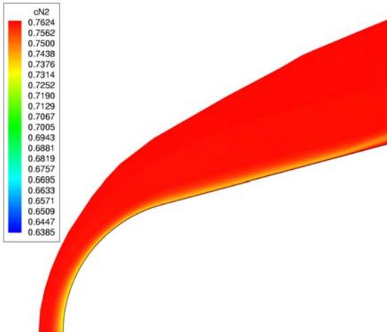
Figure 42 N<sub>2</sub> concentration at  $M_\infty=10$  for catalytic wall assumption.
